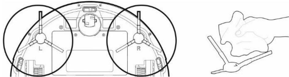
Check both side cleaning brushes together with the air intake opening according to the intensity of the contamination, at least once a week, and remove tangled hairs and other dirt.
