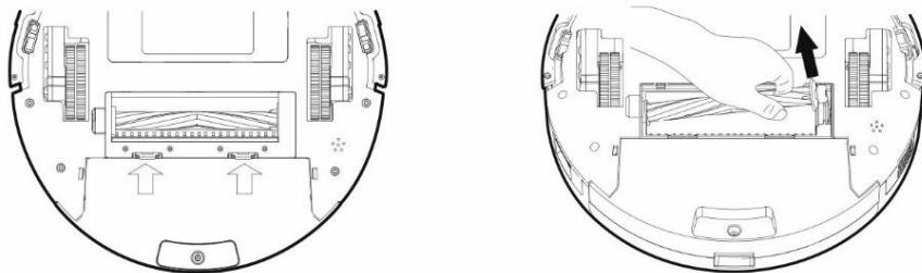
To remove the main central cleaning brush, press both tabs on the brush cover. Use a cleaning tool to remove hair entangled in the main central brush. Keep the central cleaning brush free of much hair, dust, cotton, etc.
