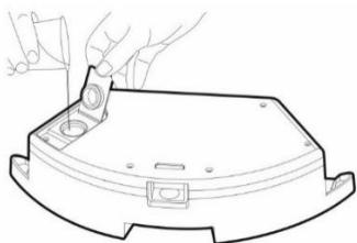
Open the plastic cap and collect water into the water tank. Only add water to the wiping container after removing the container from the vacuum cleaner.
