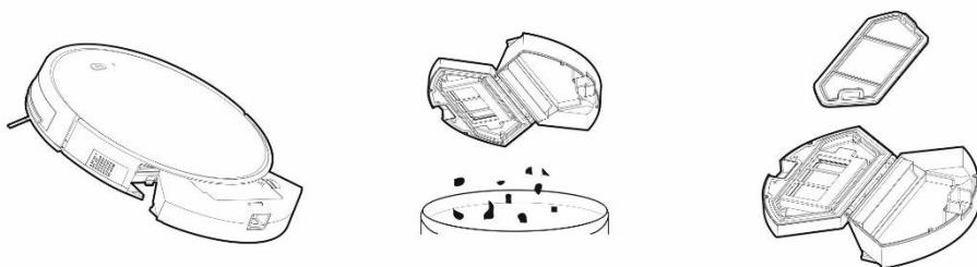
Press the release button to remove the dust tank and empty the dirt into the waste bin. We recommend washing the „Primary filter“ with clean water every 14 days.
