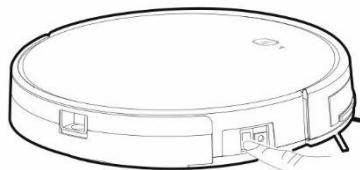
**Turn on:** set the switch button to the position **ON ( I )**
